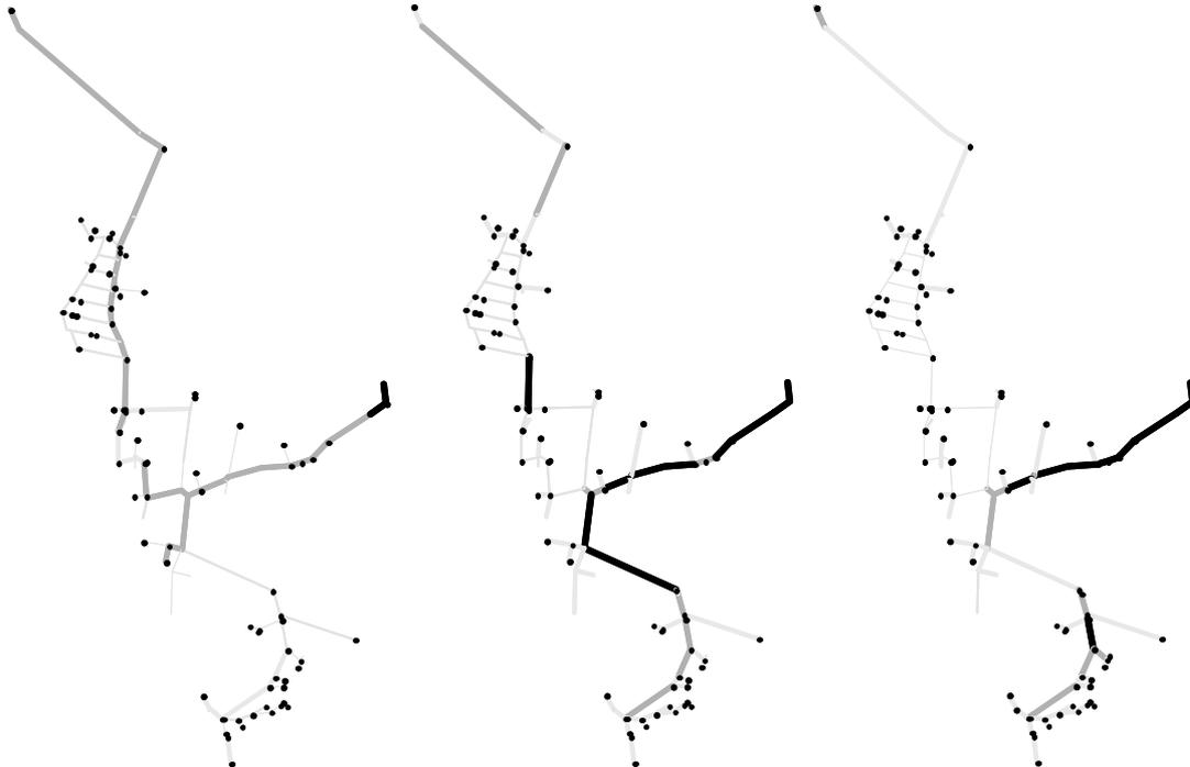
**Figure 9: Comparison of results of REL tools** (on the left : the thickness of the line represents the diameter, middle : HCI-Failnet-Reliab, without considering Predicted Failure Rate), right : HCI-Failnet-Reliab, considering Predicted Failure Rate)
